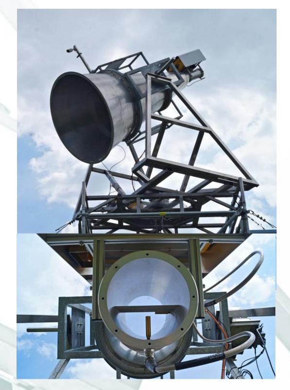
Attenuation: -3 dB beamwidth of ± 6° Detection sensitivity ~10<sup>-13</sup> W
